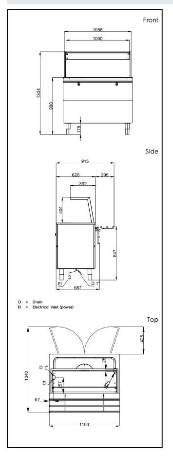
Flexy Compact Refrigerated well on cupboard, static with fan (3GN) overshelf with LED lights, H=900mm The company reserves the right to make modifications to the products without prior notice. All information correct at time of printing.
